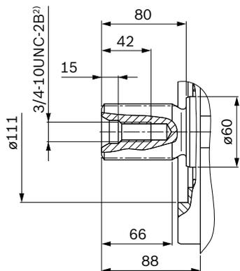
▼ Splined shaft DIN 5480
