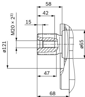
1) Involute spline according to ANSI B92.1a, 30° pressure angle, flat root, side fit, tolerance class 5
