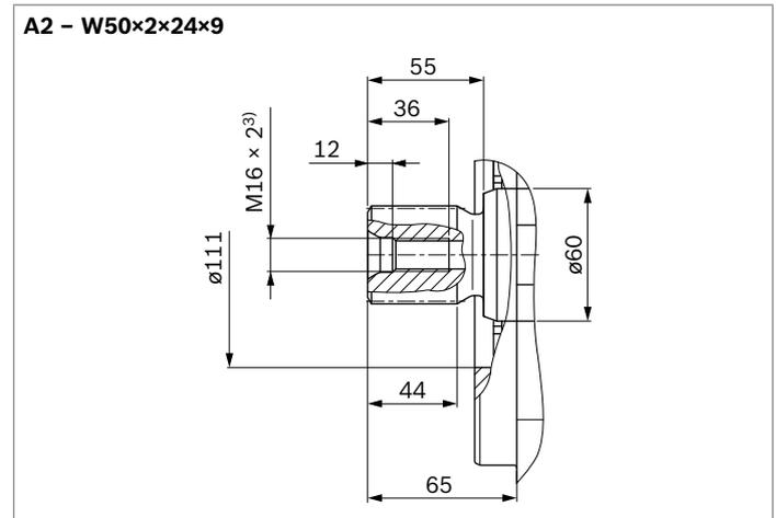
1) Involute spline according to ANSI B92.1a, 30° pressure angle, flat root, side fit, tolerance class 5
