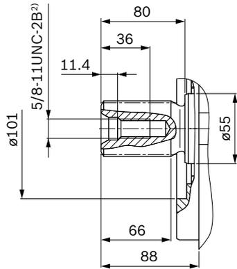
▼ **Splined shaft DIN 5480**
