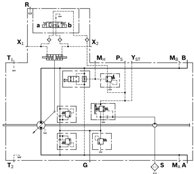
**DA..5 – DA control valve, fixed setting and brake inch valve mounted**
