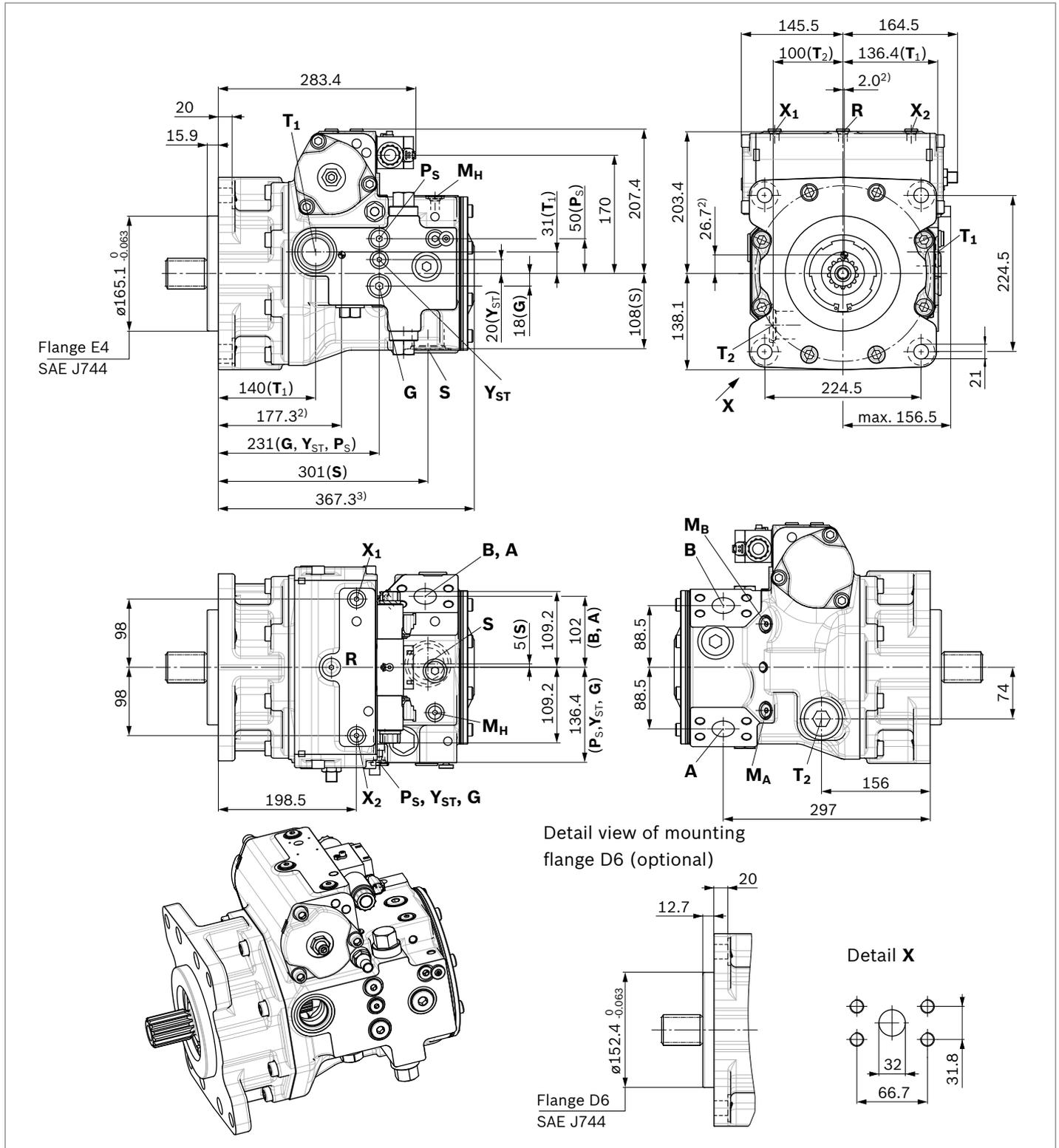
1) For SAE working ports **A** and **B**, 45° right (viewed on drive shaft), the complete case and thus the dimensions are mirrored.
