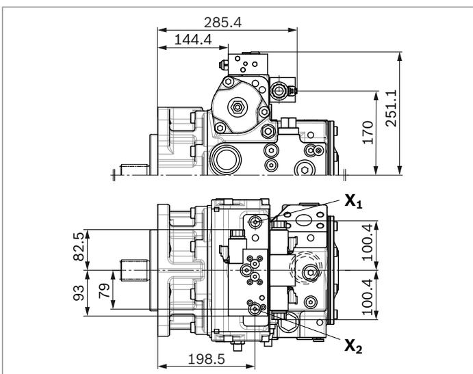
▼ **ET** – Electric control, direct operated, two DRE
