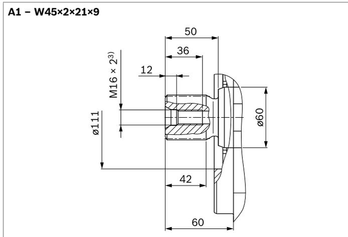
▼ **Splined shaft DIN 5480**
