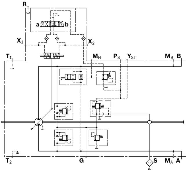
**DA..2, DA..3 – DA control valve, mechanically adjustable with position lever**
