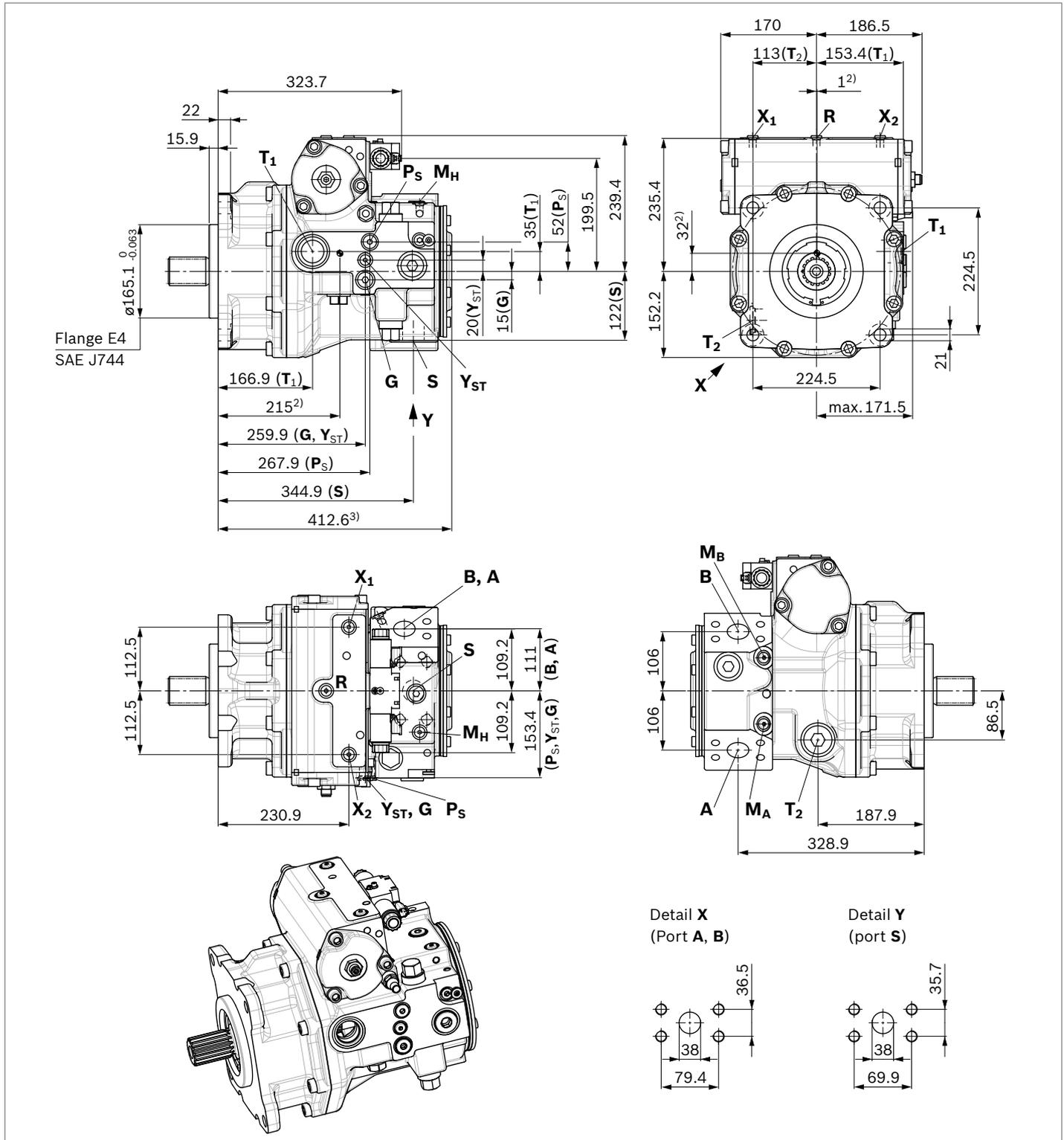
1) For SAE working ports **A** and **B**, 45° right (viewed on drive shaft), the complete case and thus the dimensions are mirrored.
