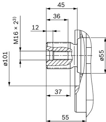
▼ **Splined shaft DIN 5480**
