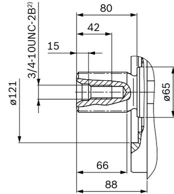
▼ Splined shaft DIN 5480
