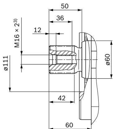
▼ Splined shaft DIN 5480
