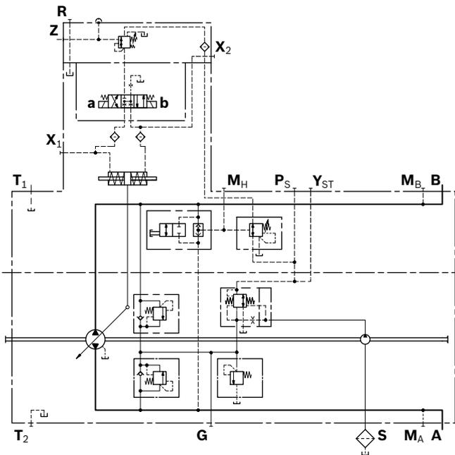
**DA..6 – DA control valve, fixed setting, ports for pilot control device as inch valve**
