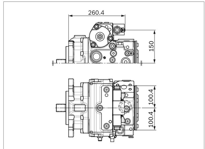
▼ **EV** – Electric control, direct operated, 4/3-way directional valve, one DRE
