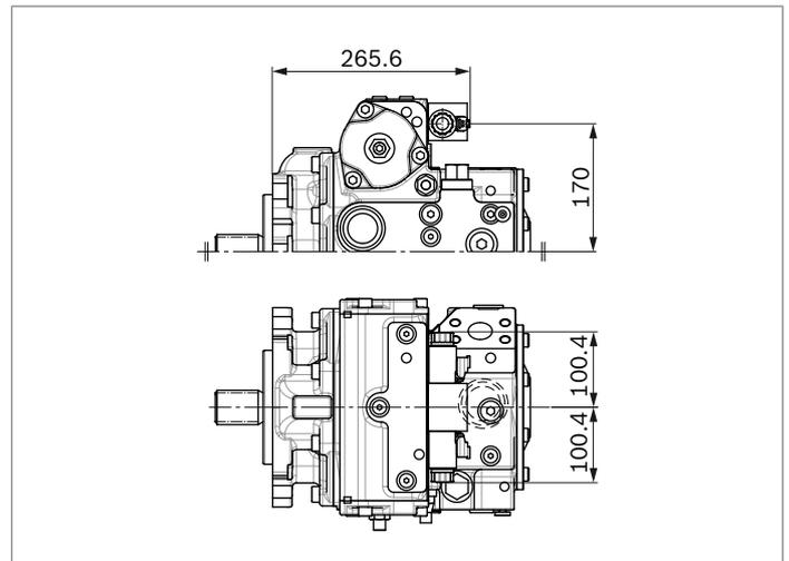
▼ **EV** – Electric control, direct operated, 4/3-way directional valve, one DRE
