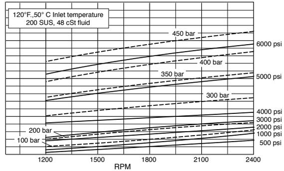
**VOLUMETRIC EFFICIENCY @ FULL STROKE**
