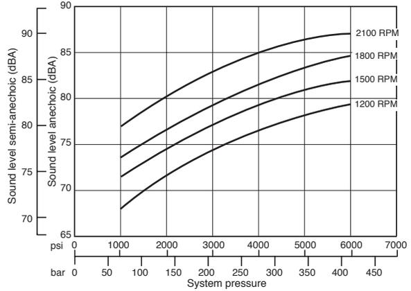
**Note:** Pump acoustical data was determined in accordance with ANSI/B93.71M, Hydraulic Fluid Power Pumps test code for the determination of airborne noise levels. Semi-anechoic values are presented according to the standard. Anechoic values are calculated for comparison with DIN 45635, part 1. The DIN standards measures sound levels over different surface areas so comparisons are not exact.
