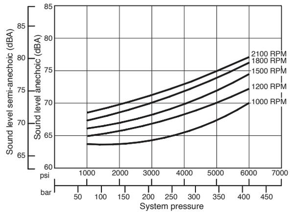
**Note:** Pump acoustical data was determined in accordance with ANSI/B93.71M, Hydraulic Fluid Power Pumps test code for the determination of airborne noise levels. Semi-anechoic values are presented according to the standard. Anechoic values are calculated for comparison with DIN 45635, part 1. The DIN standards measures sound levels over different surface areas so comparisons are not exact.
