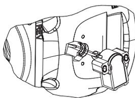
After engaging shaft slot to pin, hold sensor flush to pump pad and rotate to align screw slots to screw holes. Secure with screws & washers, 2 places.
