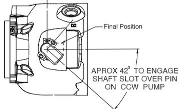
After engaging shaft slot to pin, hold sensor flush to pump pad and rotate to align screw slots to screw holes. Secure with screws & washers, 2 places.
